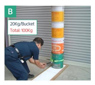
3 Pulled the stacked buckets with a spring scale.
